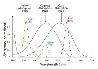
Figure 6: Absorption peak of each dye and our RGB projector emission spectrum
