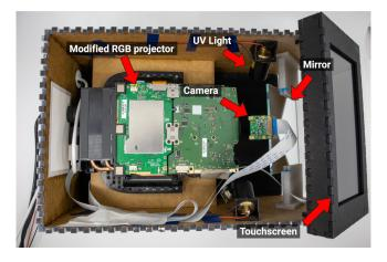
Figure 5: ChromaNails the physical prototype
