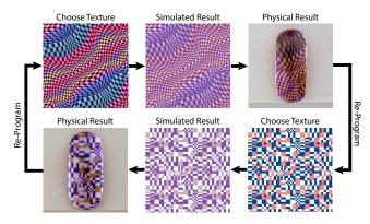
**Figure 2: The Re-programming Process**
