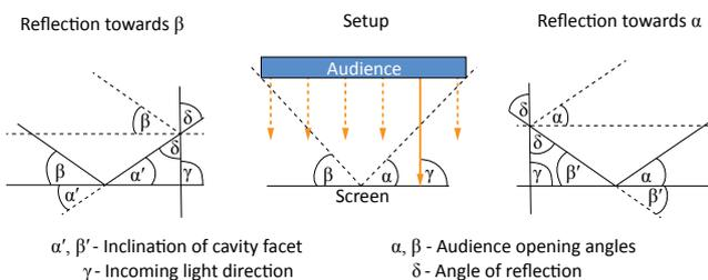
Fig. A.21. Reparameterization using the opening angle of the audience.
