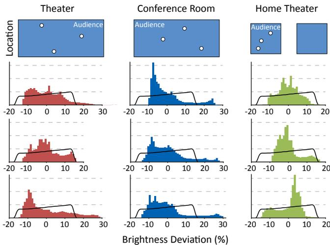
Fig. 12. We randomly sampled viewing locations in the audience (white dots). For each location a corresponding histogram shows distribution of relative brightness with respect to the mean. We compared it with a high-gain screen, shown as a black line.
