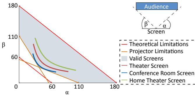
**Fig. 8.** Screen design space plot. Red straight lines mark theoretical limits of directional screens. Orange lines show the gamut of our particular screen-projector setup. Colored curves show our prototype screens. A directional screen reflects light from each point towards the entire audience. At a particular location we can parametrize this reflection by the opening angles  $\alpha$  and  $\beta$ .
