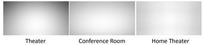
Fig. 10. Calibration masks used to equalize the brightness across each screen.
