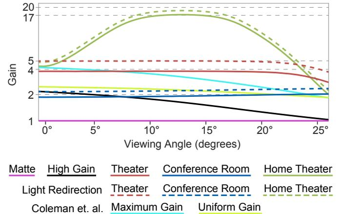
Fig. 13. Brightness (gain) of each screen relative to the brightness provided by a matte screen. Gain is presented on a logarithmic scale which better corresponds to human perception. Solid lines represent our screens with calibration performed by light attenuation, dashed lines with a projector which redirects light [8].
