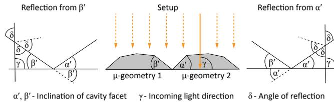
Fig. A.20. Self-shadowing parametrized with facet angle.
